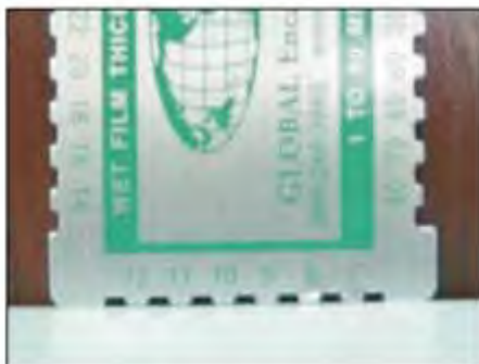
Wet Mil Gauge in Coating
